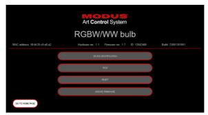
**DEVICE IDENTIFICATION:** turns on flashing white for several seconds, enabling unambiguous identification and location of the device installation location.
